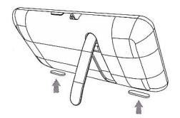
When using the bracket, the Bluetooth Speaker may wobble, even on a smooth surface. Non-slip pads can be put on the bottom edge of the Bluetooth Speaker to increase friction for additional stability.
