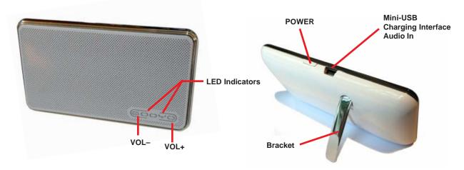
In use, it is suggested that the Bluetooth Speaker be set for maximum output volume and left that way. Use the Loudness slider in **Persona** for adjustments.
